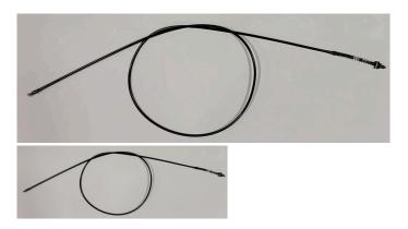
Falcon Parts Falcon Rear Brake Wire
